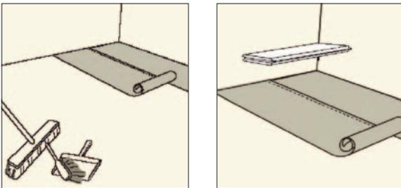
2. Roll out the underlay at 90° to the direction of the floor installation with the polythene side upwards. Peel the polythene membrane back from the wall where the first row is to be installed.
