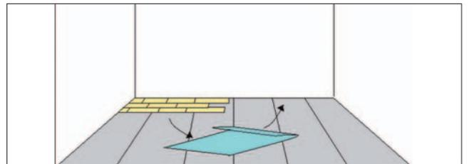
7. Install further rows by laying the planks on top of the folded membrane and once in position peel back the membrane from the underlay row by row. If you find you have removed too much of the membrane just replace it back to the previous row tight against the boards.
