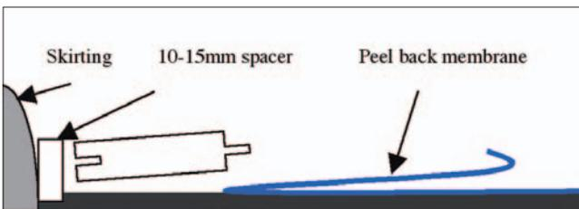
3. Now add the additional, loose membrane which can be found in the pack with the 'shiny' side face down on the adhesive. Fold the membrane with the crease facing the wall. The membrane should fold out into the room leaving enough material to take hold of after the first row has been installed.
